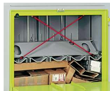
Robust: The twofold guided press ram
